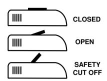
Position 3 Fully open, safety power off - Shredder not operational.
