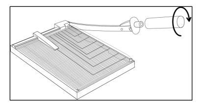
Place the guillotine on a stable flat surface. Lift the blade up to its maximum position. Place the paper on the guillotine underneath the transparent blade-guard, and then lower the blade.
