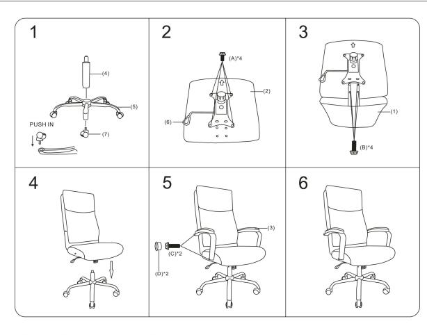
Note: Please tighten all arm screws using allen key before step 6
